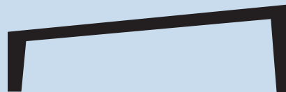
SINGLE SLOPE / MONO SLOP Practical Width : 6m - 18m
